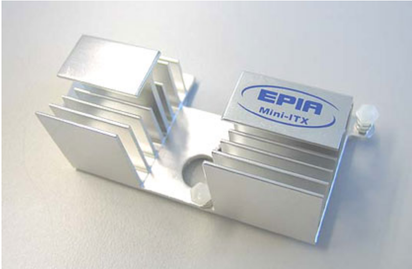
Chipset-heat sink of VIA M10000
